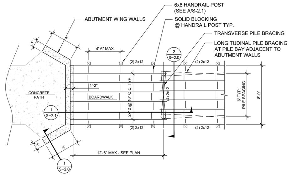
**A CONCRETE TO BOARDWALK TRANSITION PLAN**
