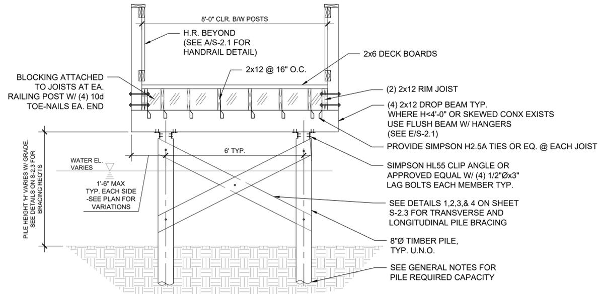
**2 TYP. BENT SECTION W/ PILES**
