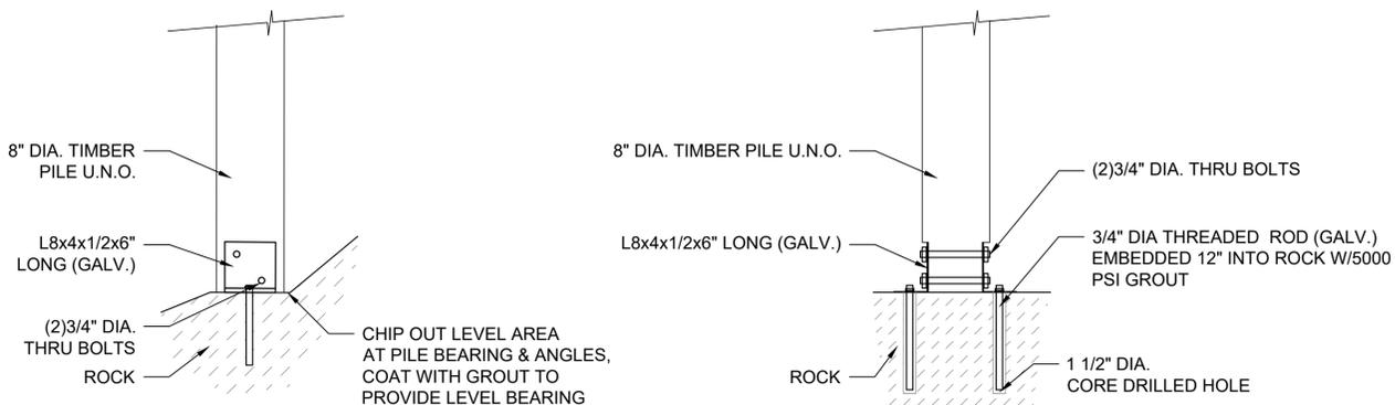
3 PILE TIP BEARING AT ROCK (ALTERNATE AT EXPOSED ROCK)
